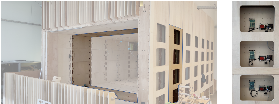
Figure 2.2: Left: The Techtile support structure – Right: The back of three tiles, equipped with the default setup, i.e. , a SDR (universal software radio peripheral (USRP) B210), processing unit (Raspberry Pi 4) and power supply with power-over-Ethernet. Each tile is connected to the central unit with an Ethernet cable, providing both power and data.
