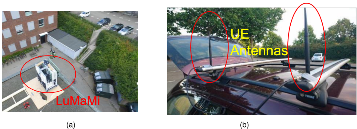
Figure 2.9: (a) LUMaMi on the roof top facing the parking lot for mobility test. (b) UE antennas mounted on top of the car roof.
